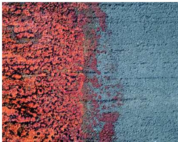
Figure 2.4 Formation of General Corrosion
