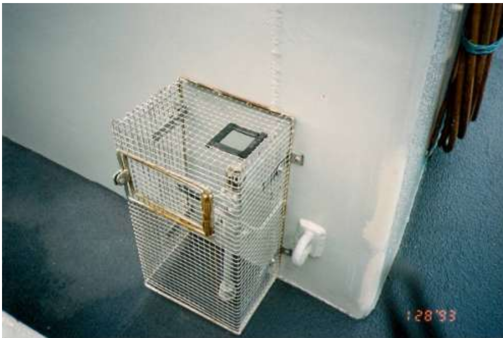
Figure 3.4 Plasticised Wire Mesh Breaking Down With Use
