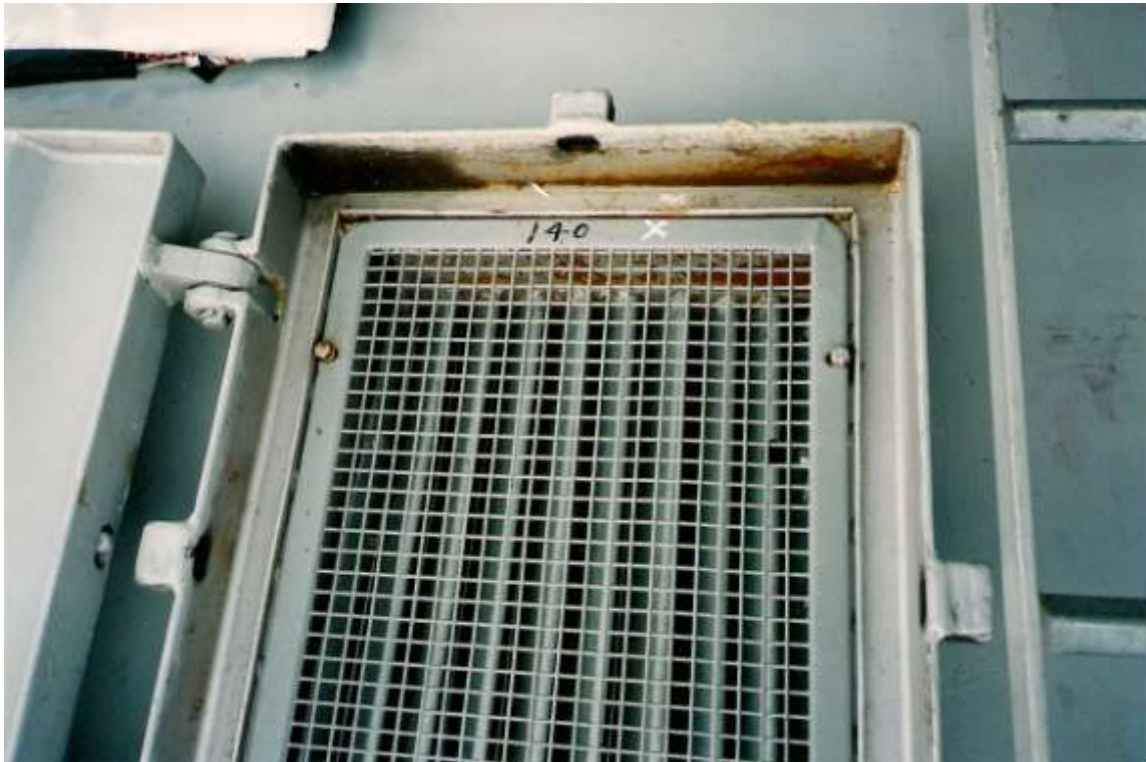
Figure 3.7 Jalousie Housing with No Gasket (note that FRP Jalousie is not corroding)
